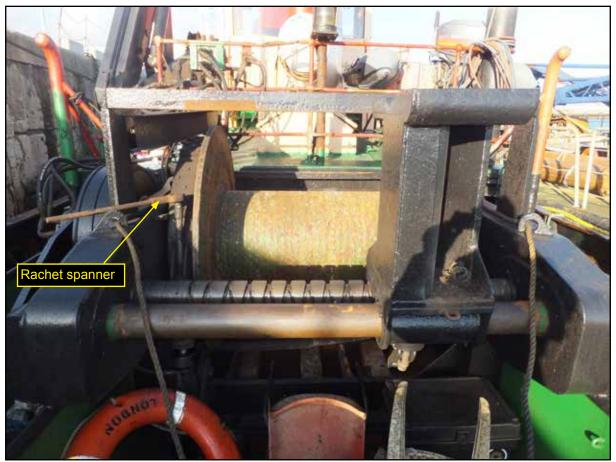
Figure 14: Kingston - towing winch
