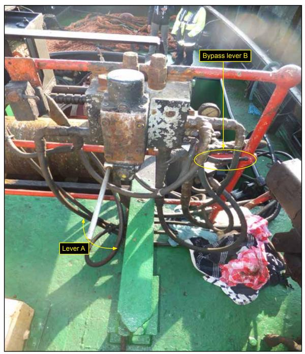
Figure 15: Kingston - towing winch hydraulic controls
