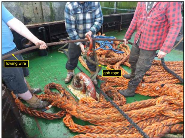
Figure 13: Kingston - gob rope arrangement
