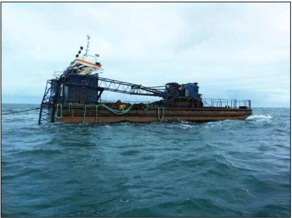
Figure 4: Walcon Wizard - collision damage
