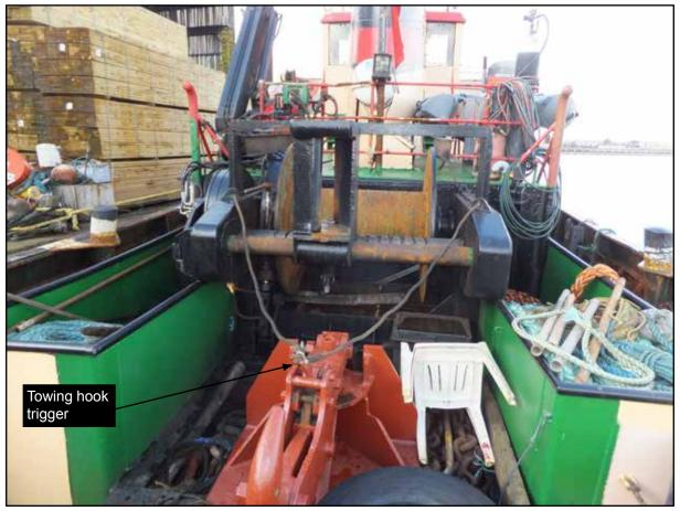
Figure 12: Kingston - towing hook release arrangement
