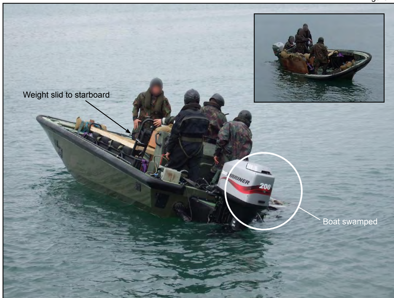
Rigid raiding craft (Mk 2) capsizing trial conducted for the Army
