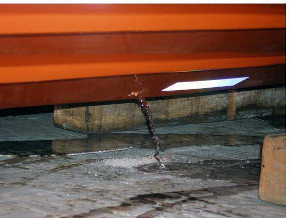
Water draining from foam-filled compartments
