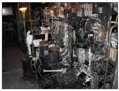
As part of the fire-fighting effort, the fixed total flooding system (high expansion foam) was activated but did not extinguish the fire. Although all of the foam solution in the system was deployed into the auxiliary engine room, no foam was produced. The fire burned fiercely for over 1 hour before it was extinguished by the ship's crew.
