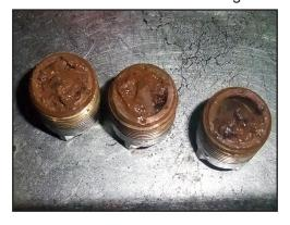
• The distribution pipework for the foam solution contained debris and was corroded (Figure 3).
