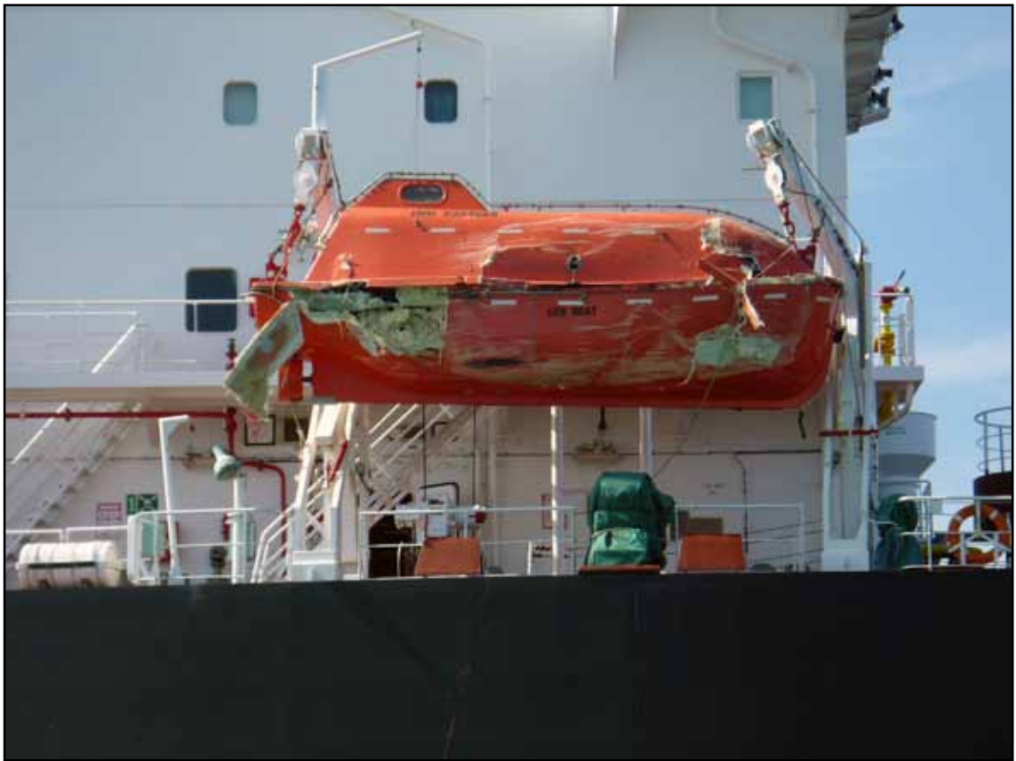
Damage to Saetta's starboard lifeboat
