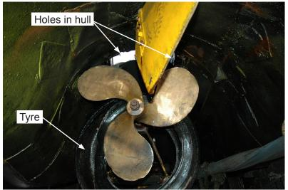
Figure 1: Holes torn into WQ1's hull after the propeller was fouled by a tyre
