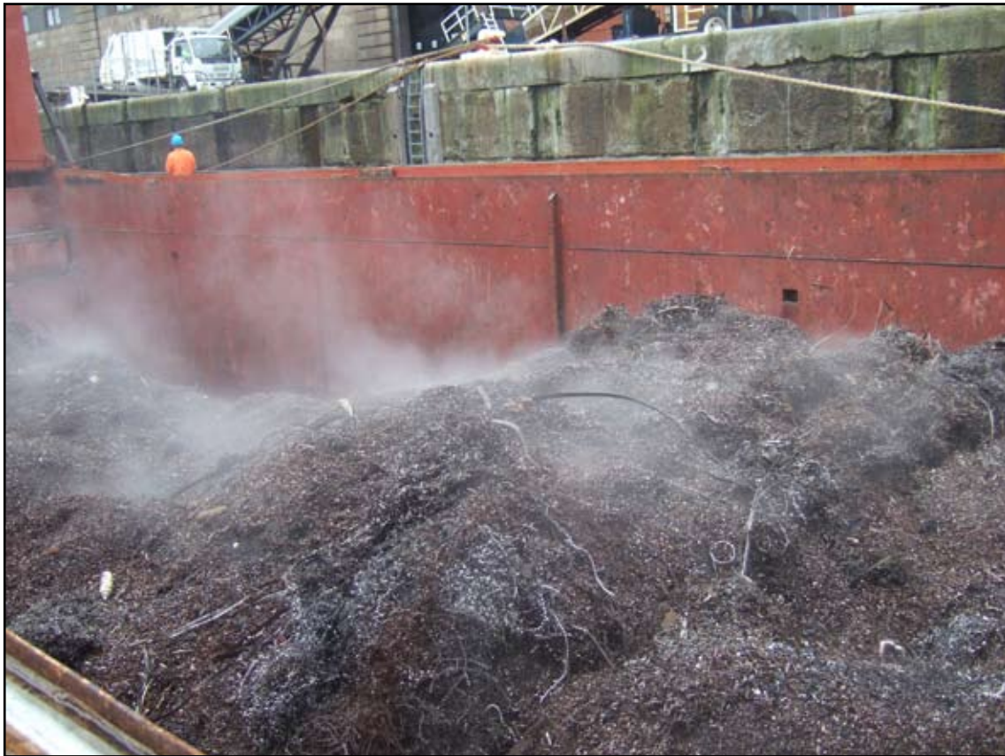
Steel turnings on board Sava Lake (as photographed in Dover on 19 January 2008)
