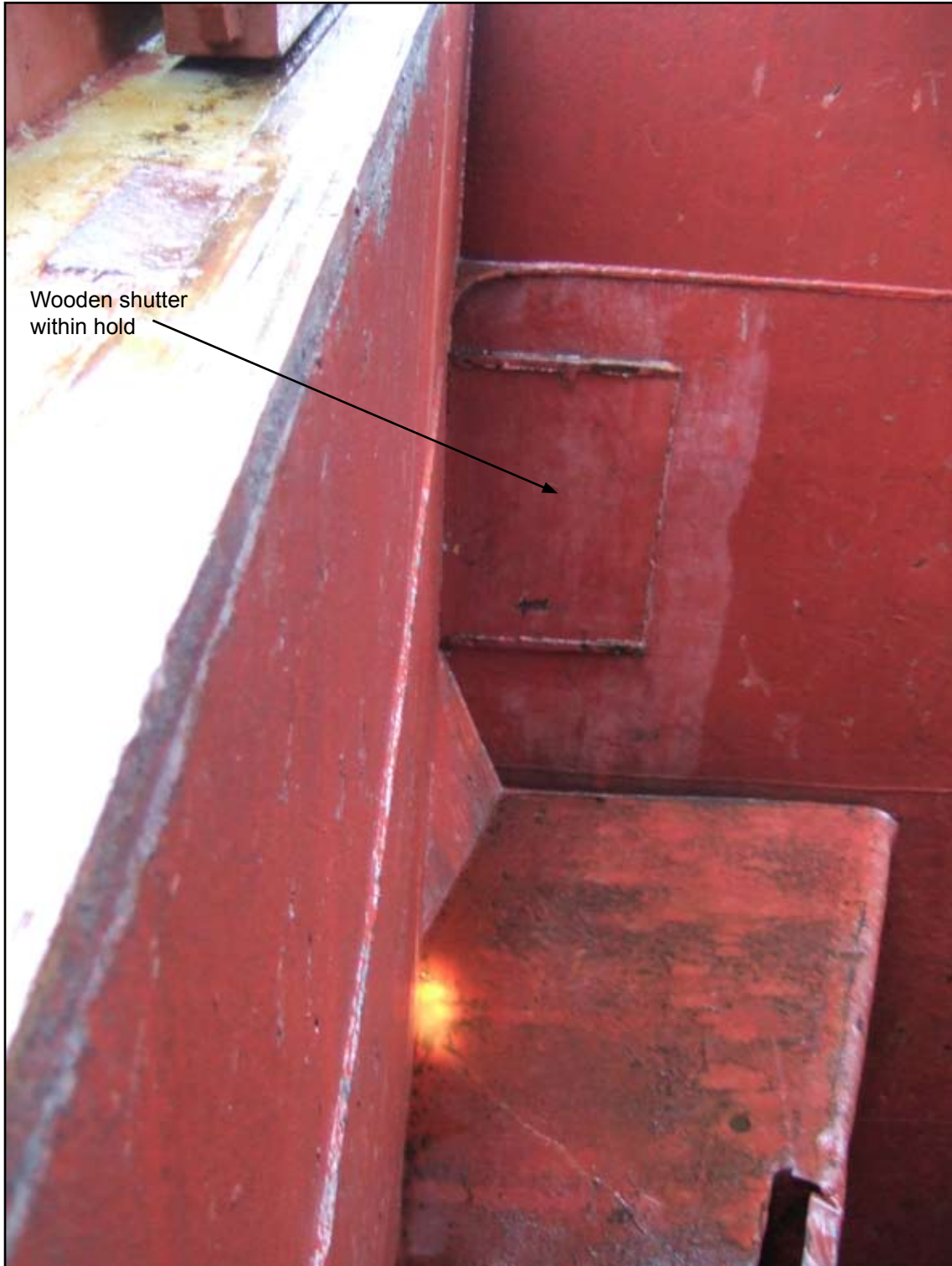
Wooden shutter to cargo ventilation system - port forward cargo hold
