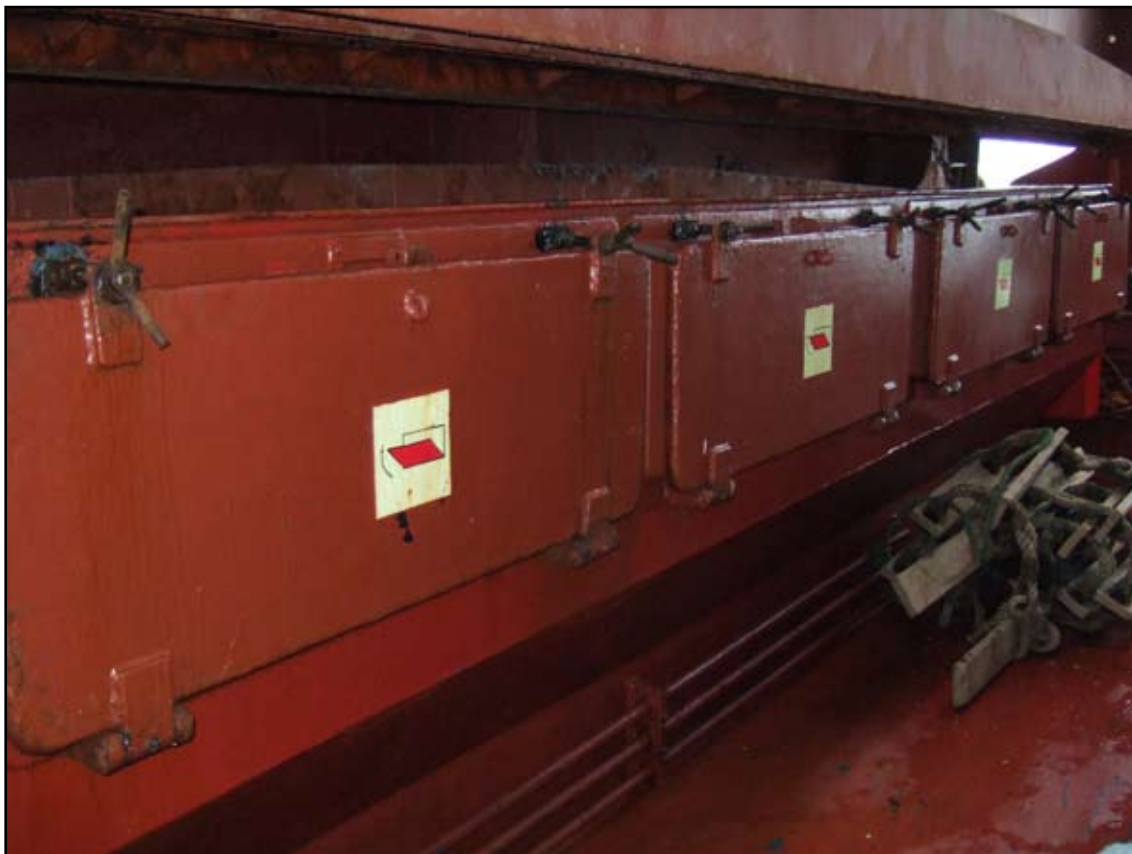
Aft cargo ventilation flaps on deck
