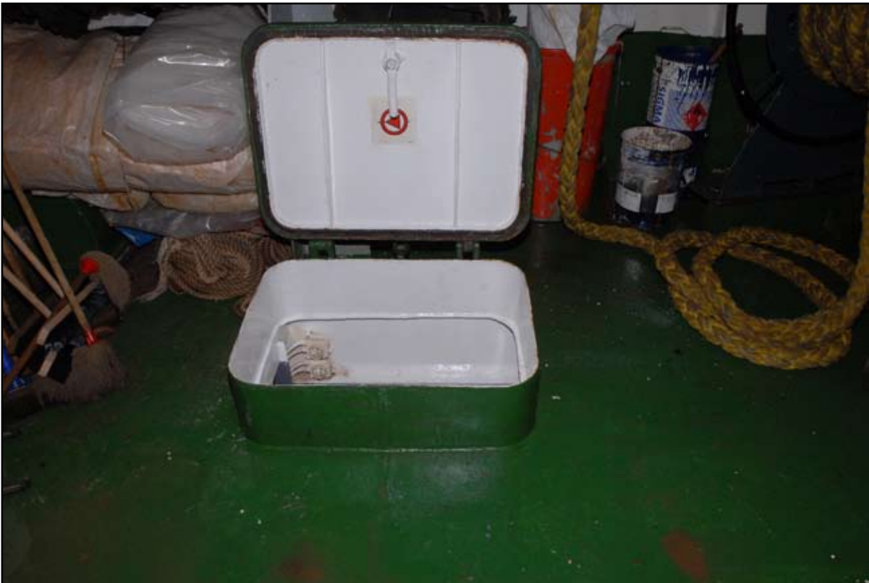
Hatch from forward store to bow thrust room
