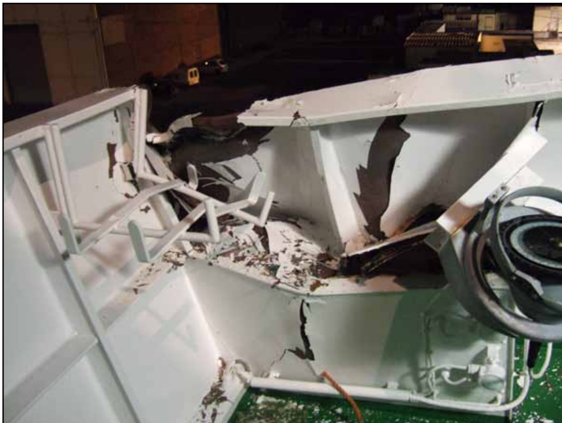
Scot Isles - damage to starboard bridging
