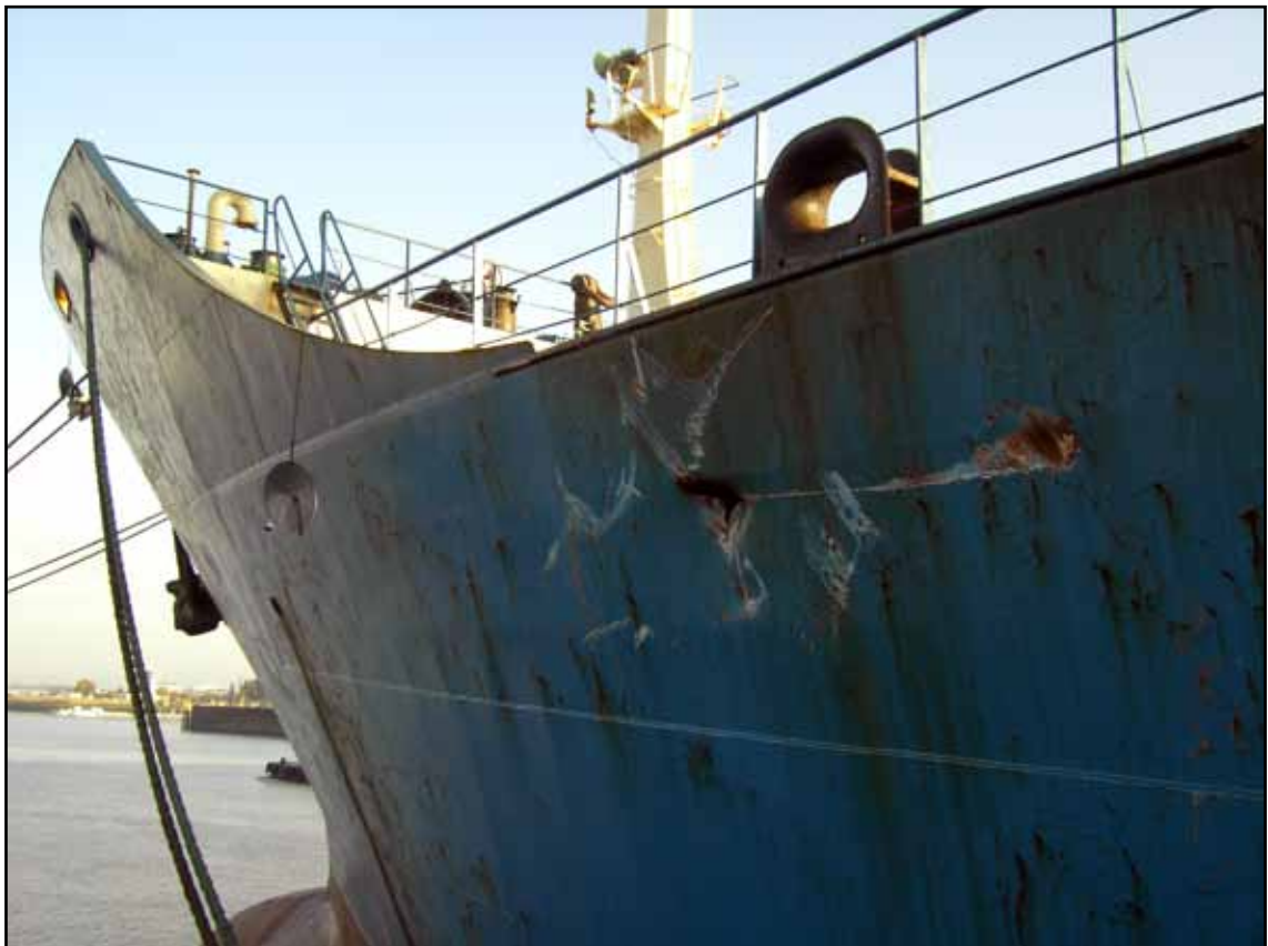
Wadi Halfa - shell plate damage to number one port wing ballast tank
