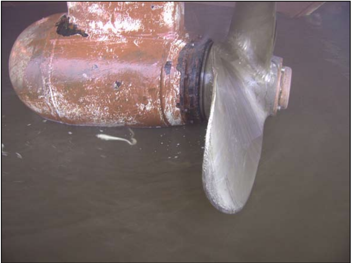
Port azimuth pod and damaged propeller
