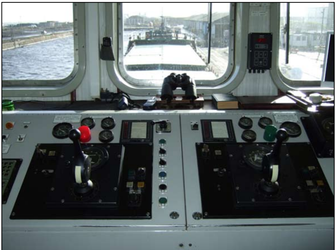
Sea Mithril's wheelhouse azimuth pod controls
