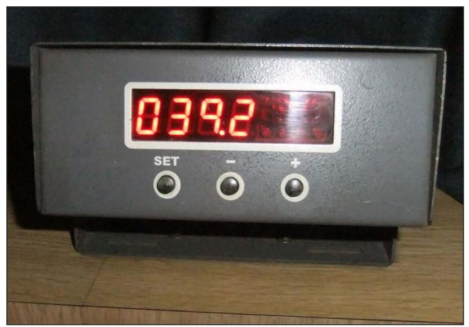
Figure 22: Timor Stream's gyro interface repeater
