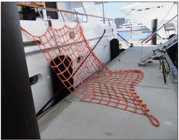
Figure 11: Battered Bull's manoverboard recovery net
