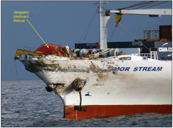
Figure 15: Timor Stream's bow section - post-collision
