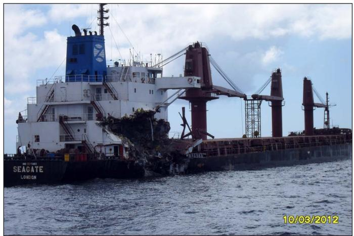
Figure 13a: Seagate's starboard side - post-collision
