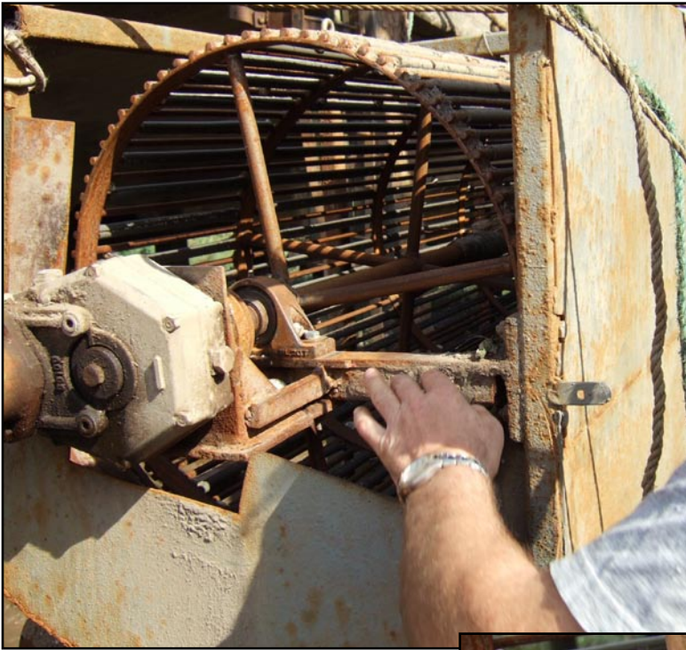
Sequence showing how the crewman's arm was caught in the shear trap
