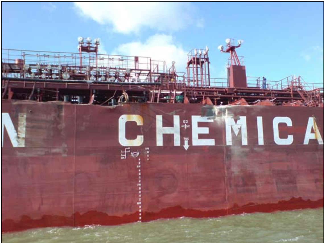
Damage to Sichem Melbourne 's sheer strake and deck edge
