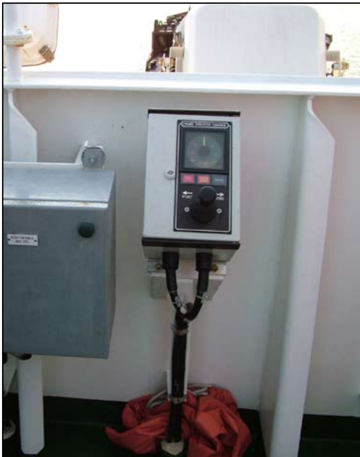
Detail of bow thruster control
