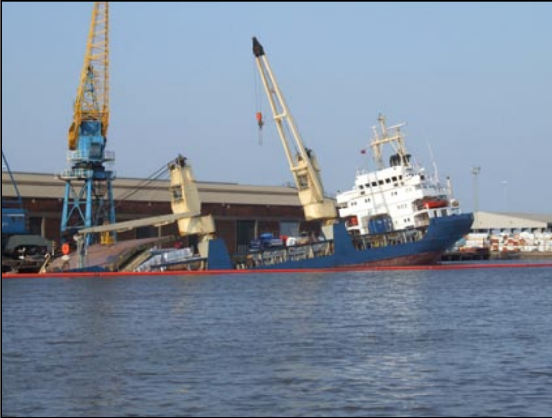
Skagern's bow settled on dock bottom
