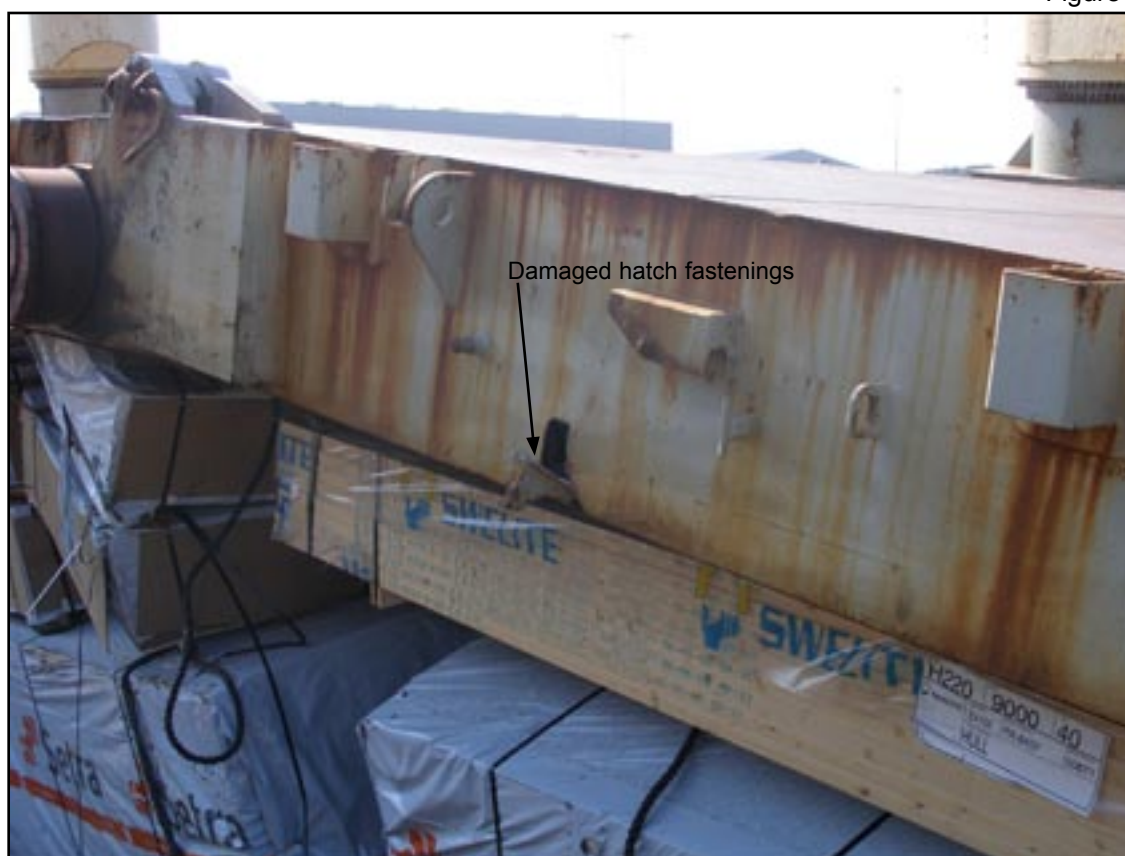
Skagern's hatches forced up by pressure of floating cargo
