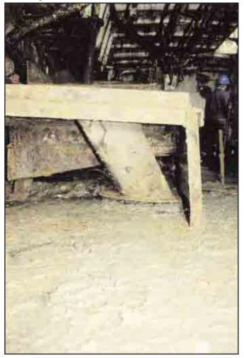
Photographs showing the gap between the deck and the flange on the starboard picking tray
