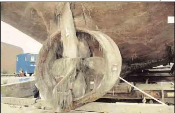
Salvage damage to kort nozzle and rudder
