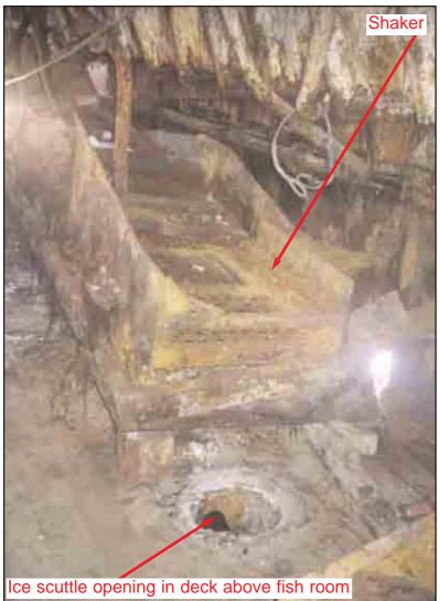
The port and starboard ice scuttles were open (Figure 10 - port scuttle shown). One of the watertight covers was found among the pile of loose gear on the starboard side, between the shaker and the wash room. The other was not found. Another securing key for the ice scuttles' covers was in the small wash room.
