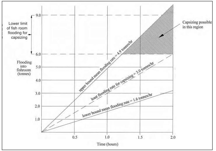
Flooding of the fish room - equating possible flooding rates and time frames
