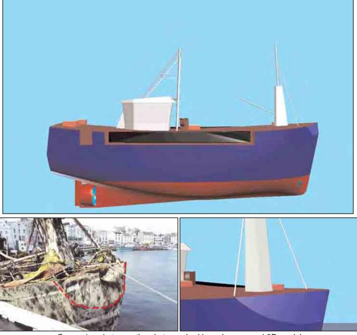
Comparison between the photographed bow damage and 3D model
