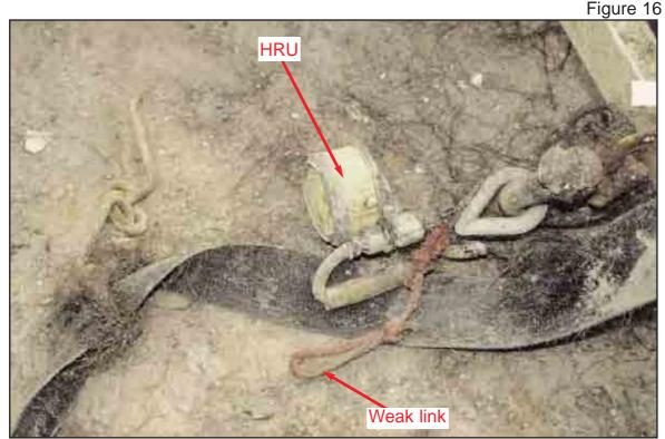
The aft liferaft securing straps and HRU
