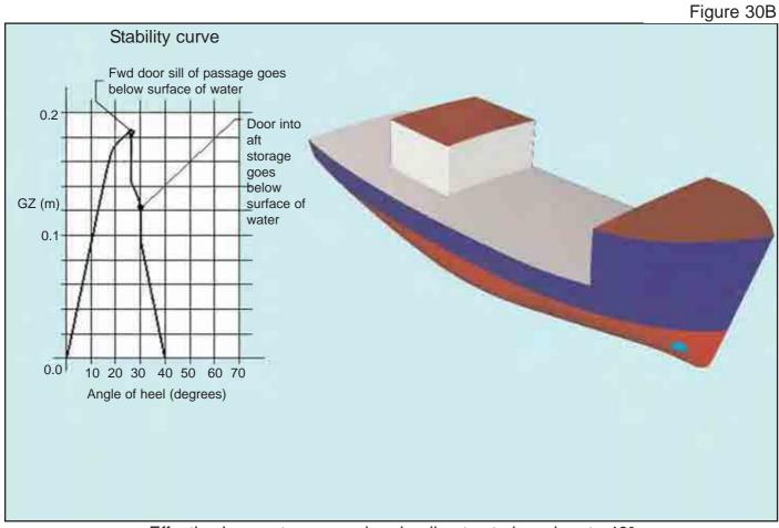
Effective buoyant spaces when heeling to starboard up to 40°
