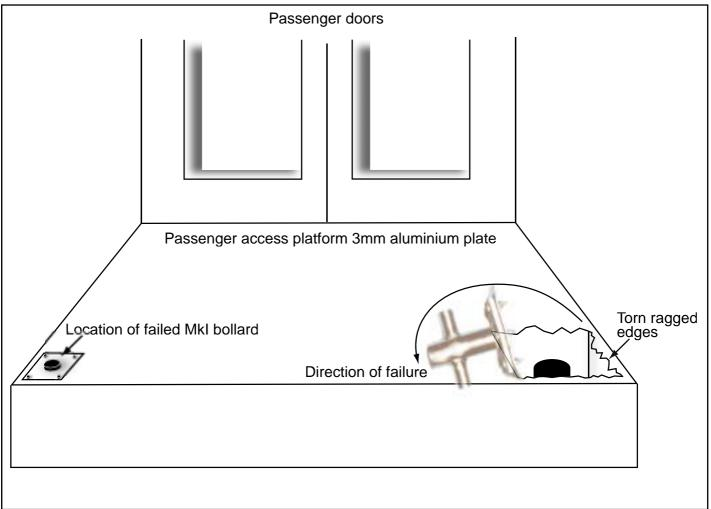
Damage to bollard arrangement sustained on 9 April 2004
