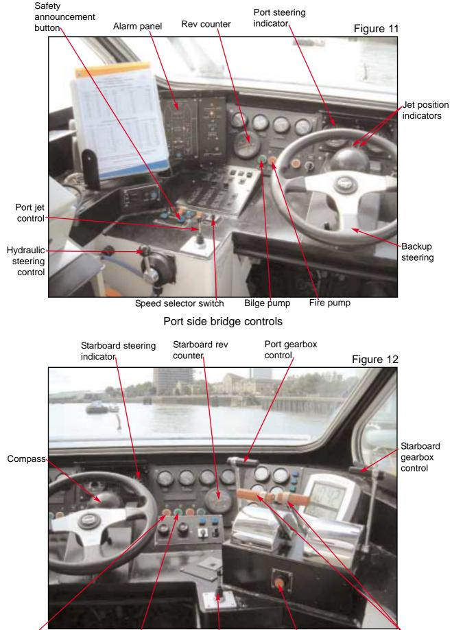
Engine start button Engine stop button Starboard jet control Ship's horn
