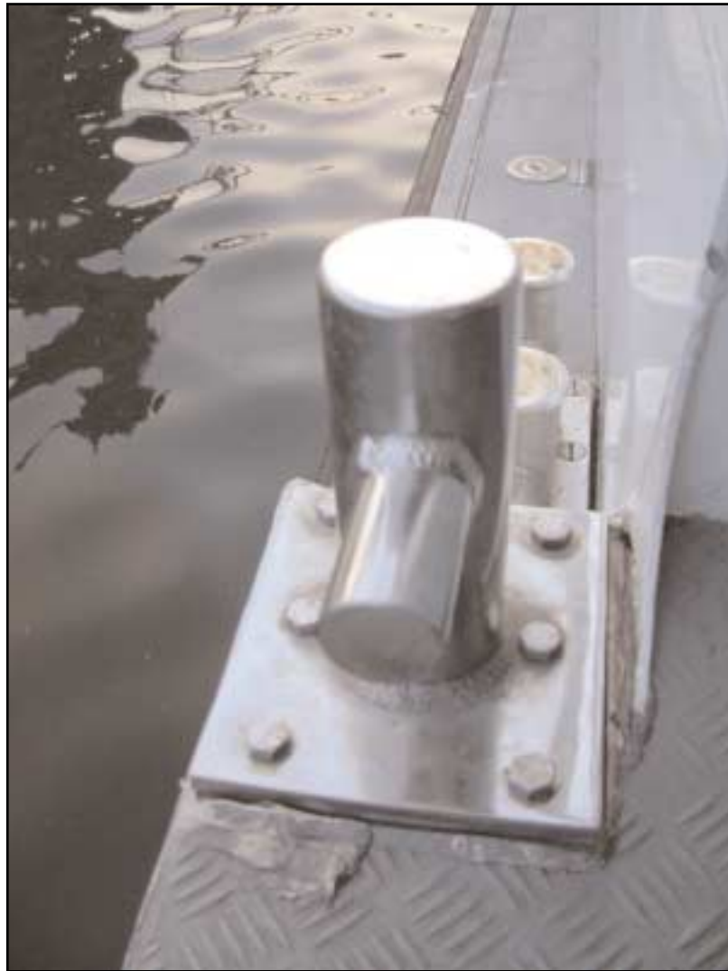
Passenger access - stainless steel MkIII bollard
