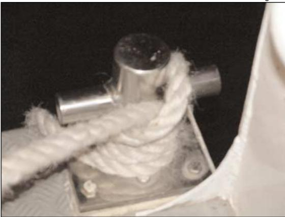
Mooring rope 'pin hitch' arrangement
