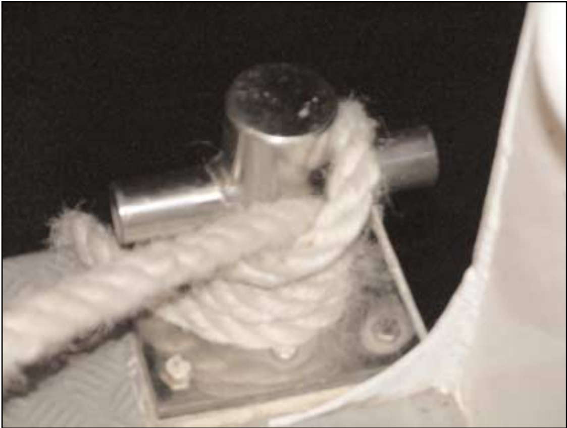
Mooring rope 'pin hitch' arrangement
