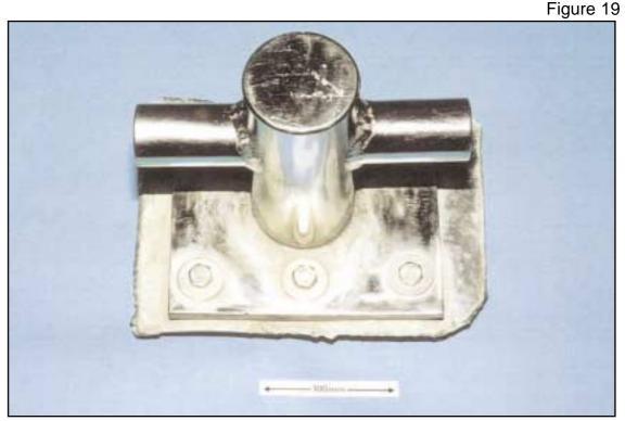
Bollard and insert plate fastening arrangements viewed from inboard side
