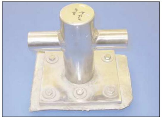
Displaced stainless steel mooring bollard and insert plate
