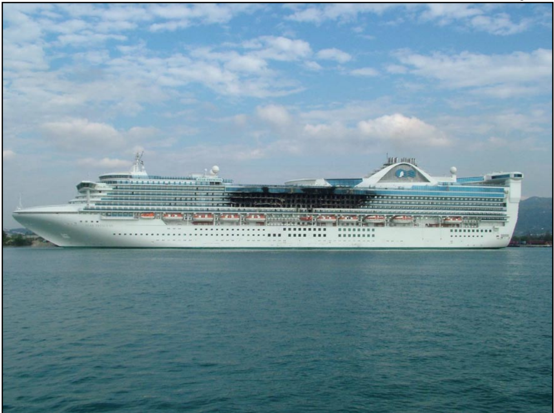
Extent of damage on ship's port side
