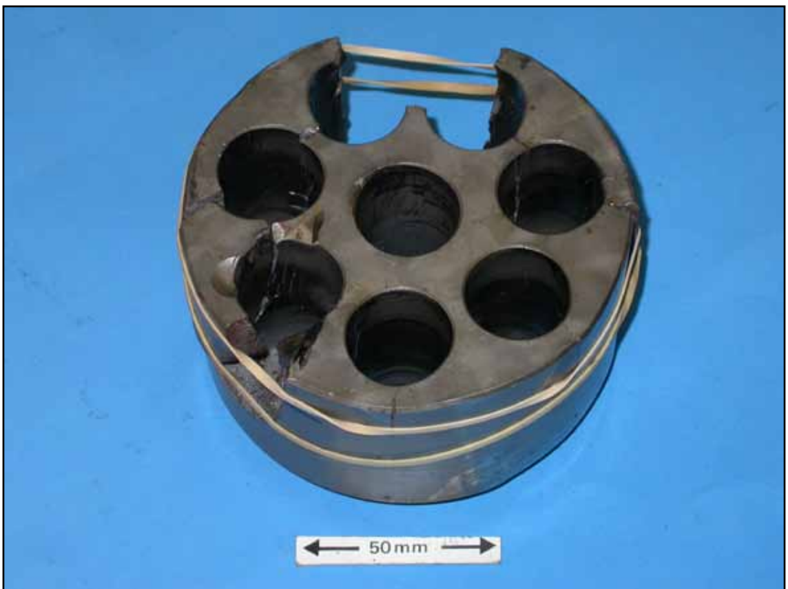
Predominant damage on one side of the cylinder housing
