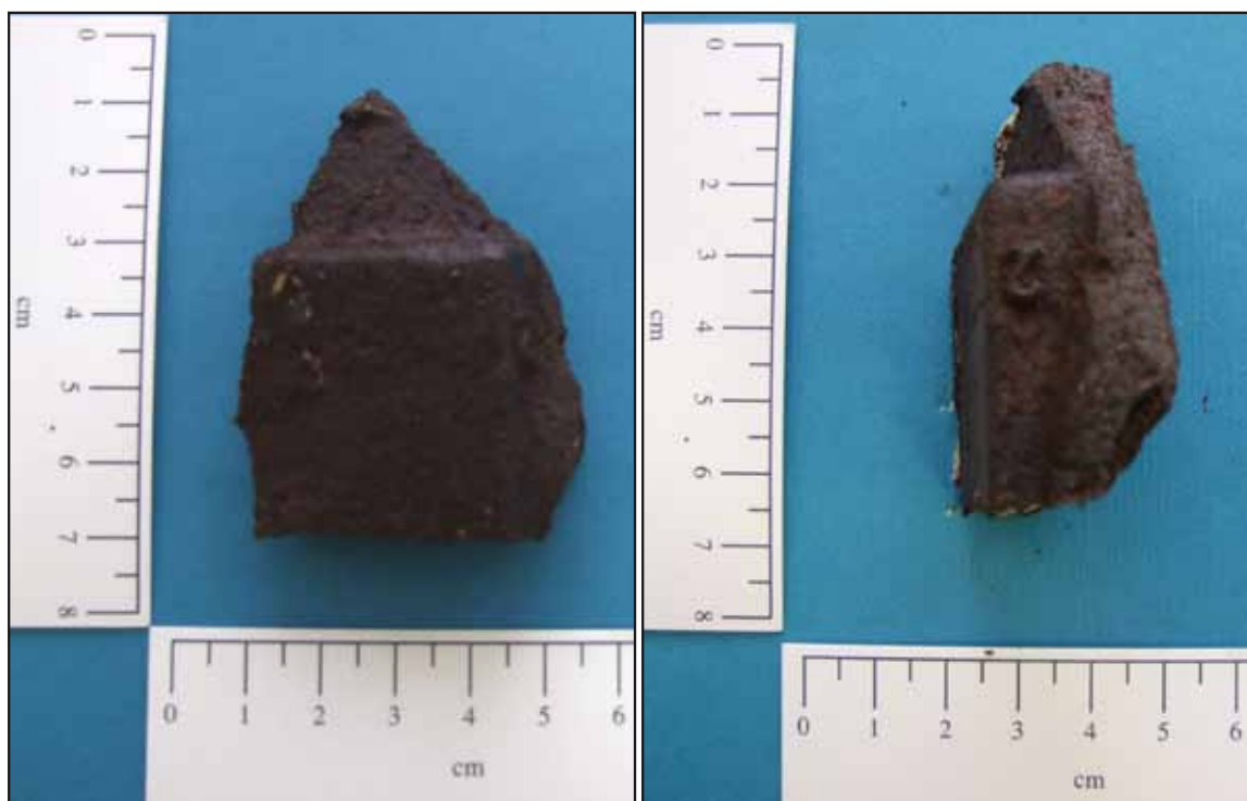
Fragment of hydraulic motor casing found 40m aft of the starboard windlass
