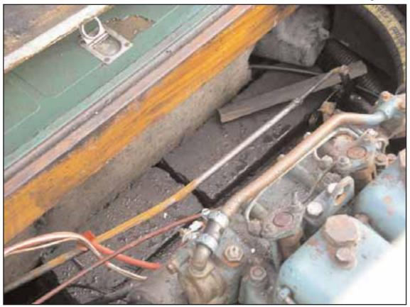
Kerbstones positioned in engine compartment
