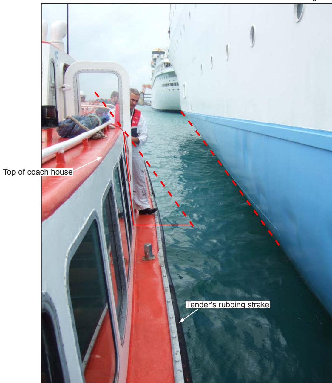
Photograph showing the curve of the ship's side at the position of the accident (dotted parallel lines indicate the coach house will strike the vessel's hull before the tender's rubbing strake)
