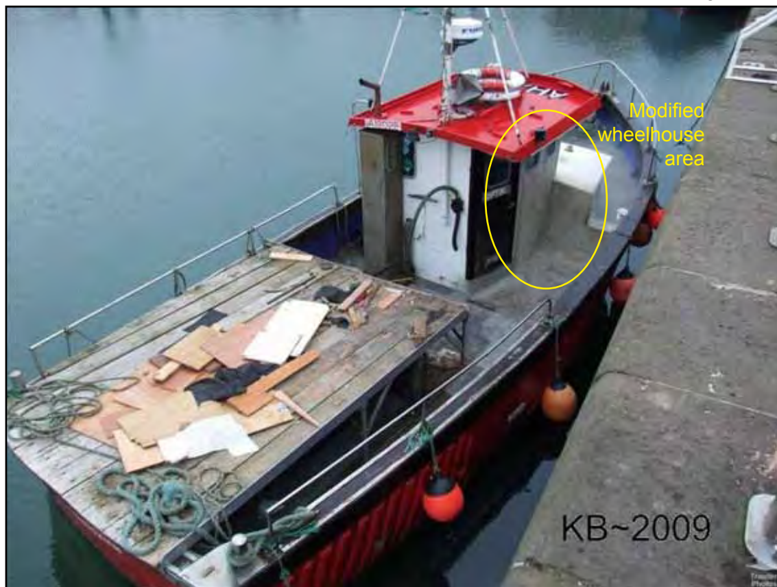
Optik undergoing modifications to starboard side of wheelhouse to enlarge deck space
