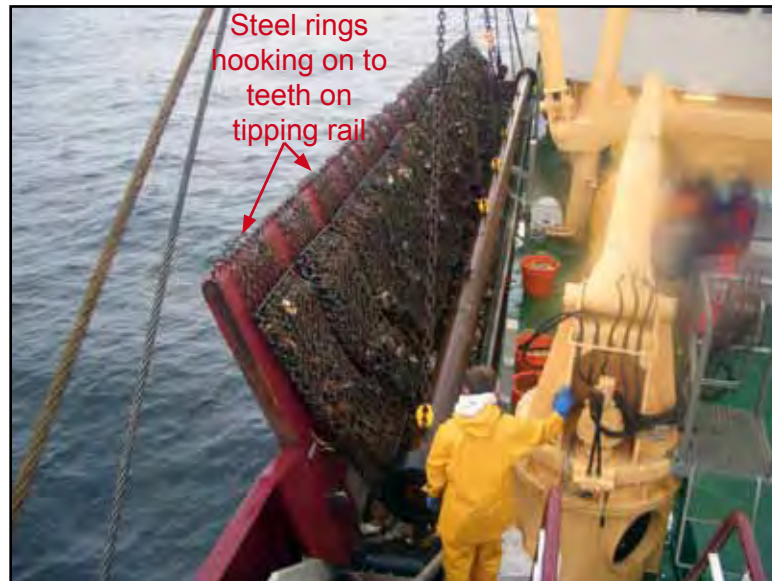
Tipping rail mechanism
