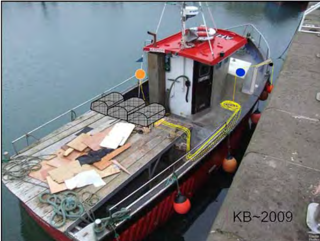
Representation of back rope coiled under the hauler and initial sequence of creels stowed on the shooting table
