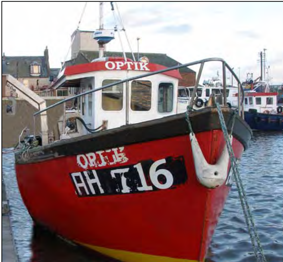
Optik showing completed modifications to wheelhouse and davit arm
