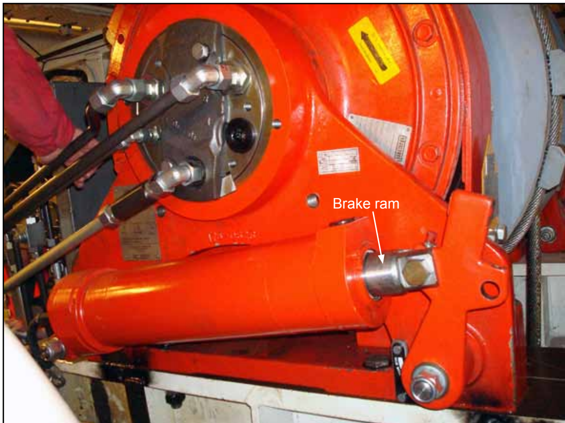
Cursor winch forward brake ram
