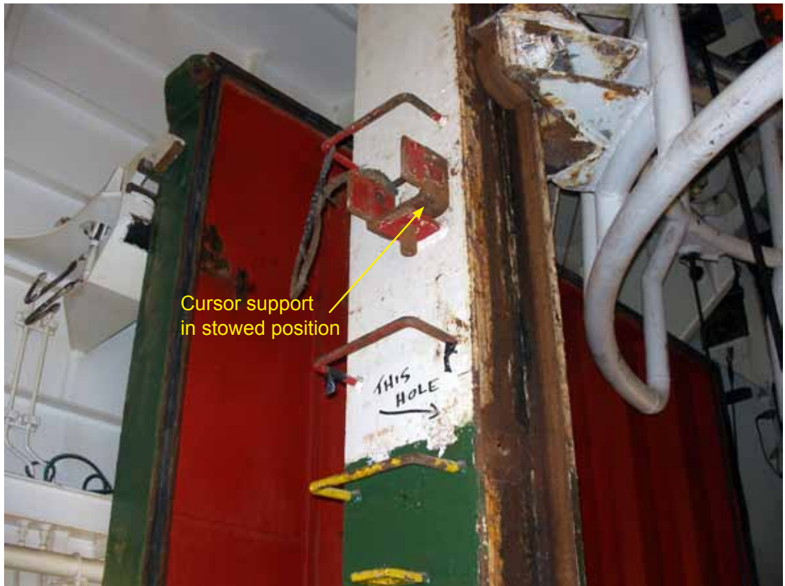
Cursor support position at the time of accident
