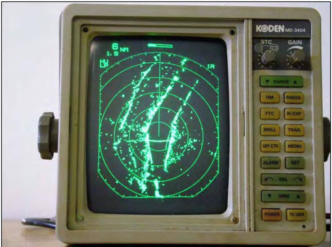
Whispa's radar screen, showing 1.5 mile range rings and oblong screen
