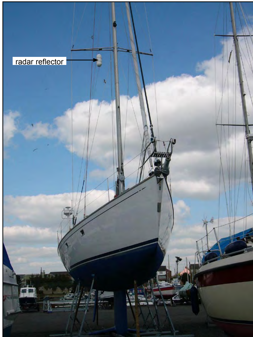
Whispa's radar reflector and mast
