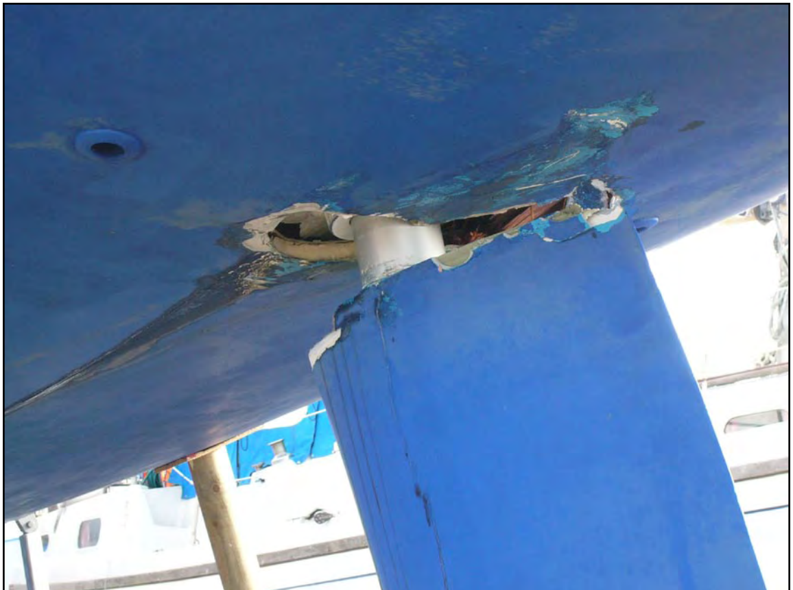
Damage to hull above rudder
