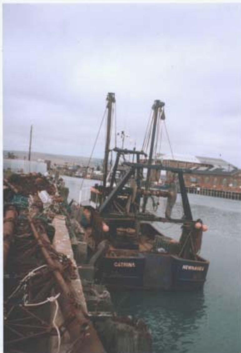
Catrina in Port, Showing Obstructions to Freeing Ports
