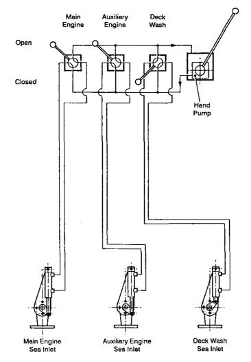
Figure 2 - Remote Operation of Seacocks
