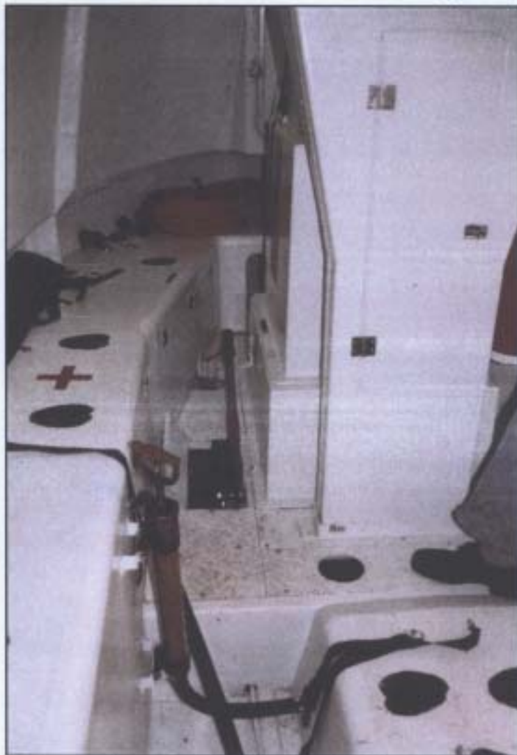
General view of inside starboard lifeboat showing difficult access to operating gear
