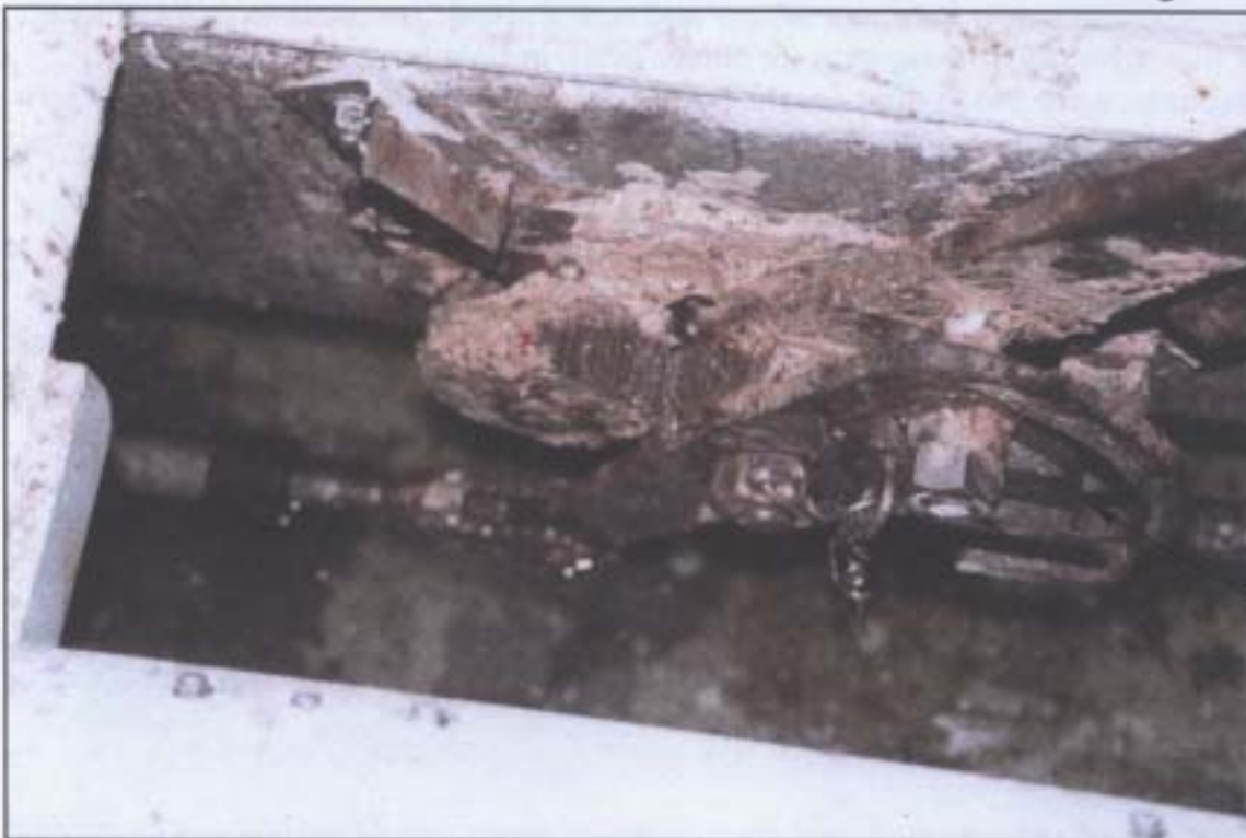
Close-up view of release gear showing quadrant in reset position but locking pin in released position
