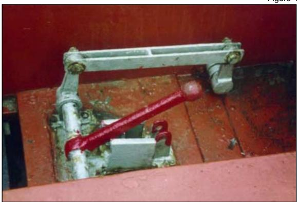
The releasing lever raised 30° from its horizontal position
