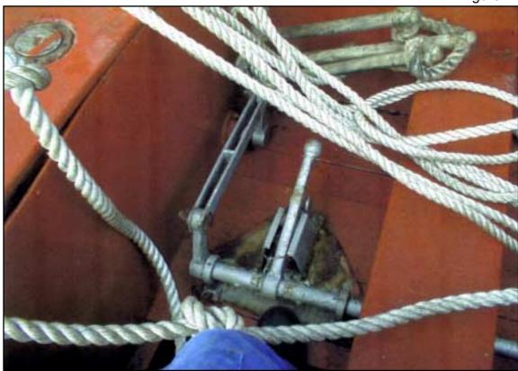
Releasing lever with safety pin missing
