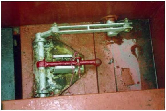
Safety pin in place to secure the releasing lever
