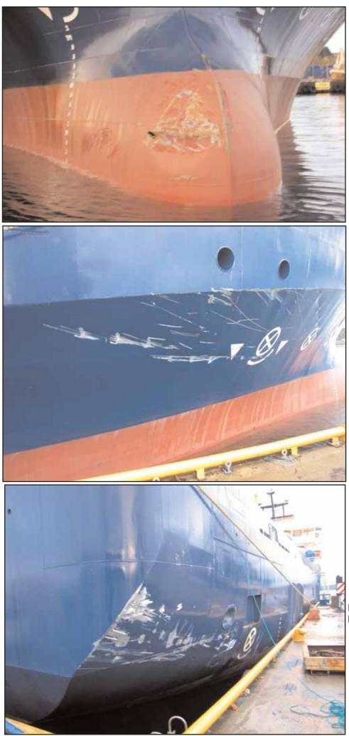
Figure 5a Damage to *Strilmøy*'s bulbous bow
