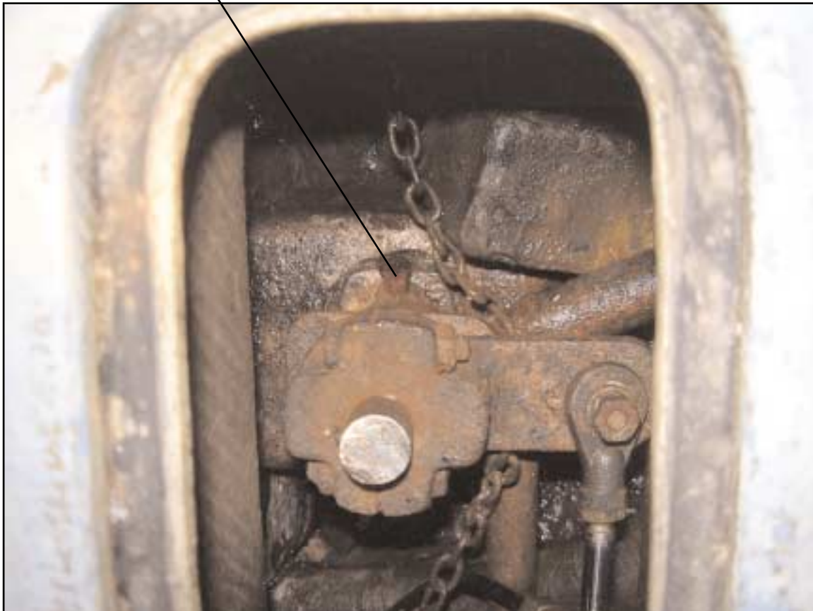
Photograph showing a wooden bung in the rudder stock
