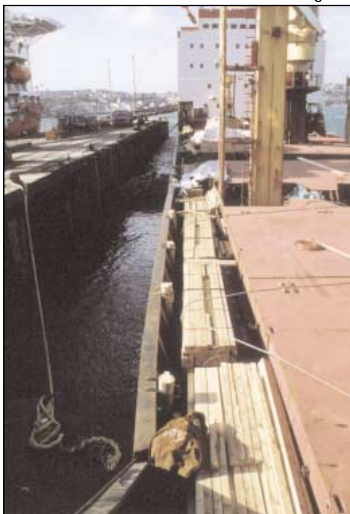
Photograph showing packages placed between the bulwark and hold hatch covers
