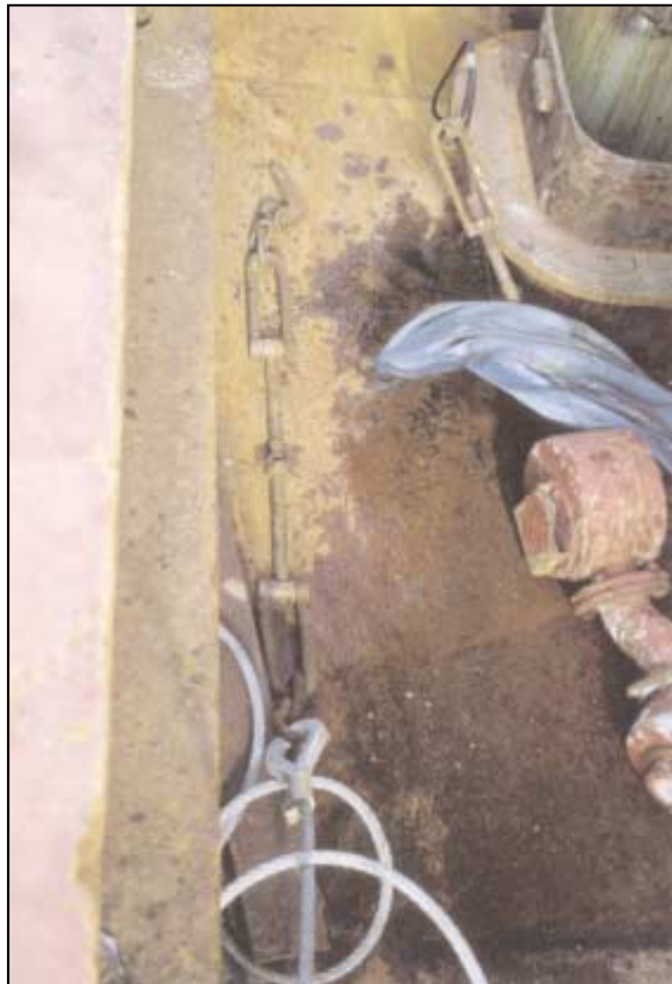
Photograph showing wire lashing with turnbuckle and pelican hook
