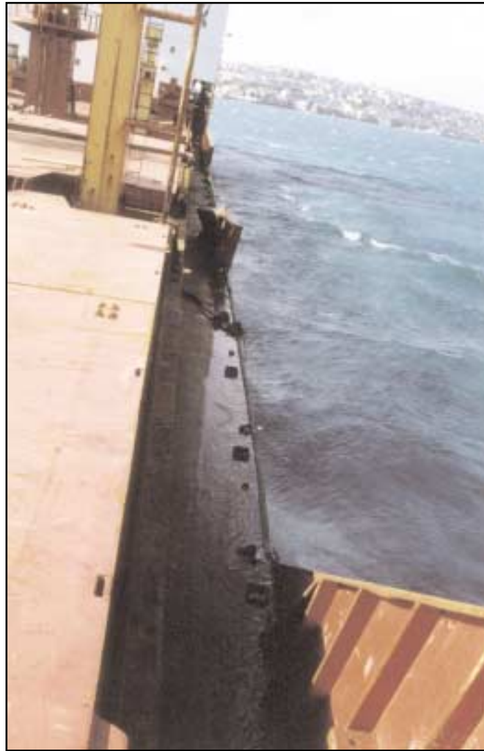
Photograph showing damage to port bulwark
