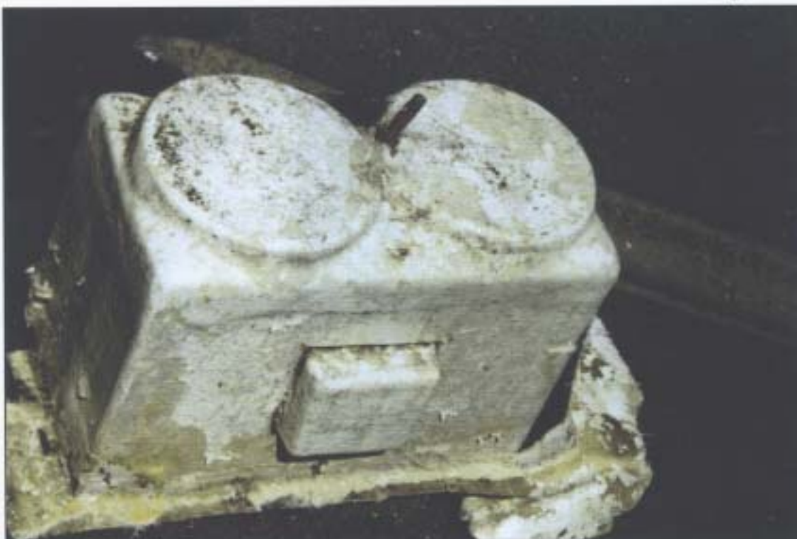
Ready-use gas bottle locker moulding following accident
