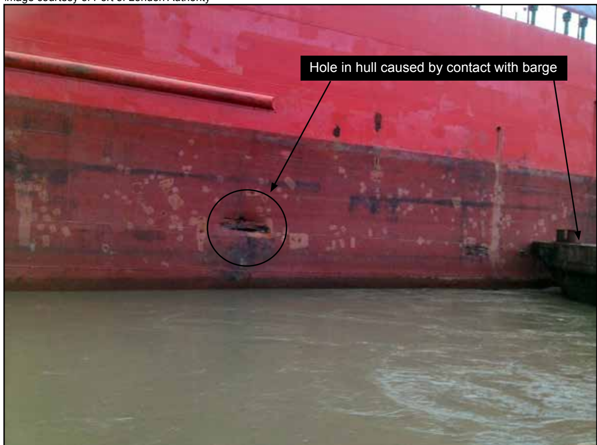
Figure 6: Shell plating damage to Amber
