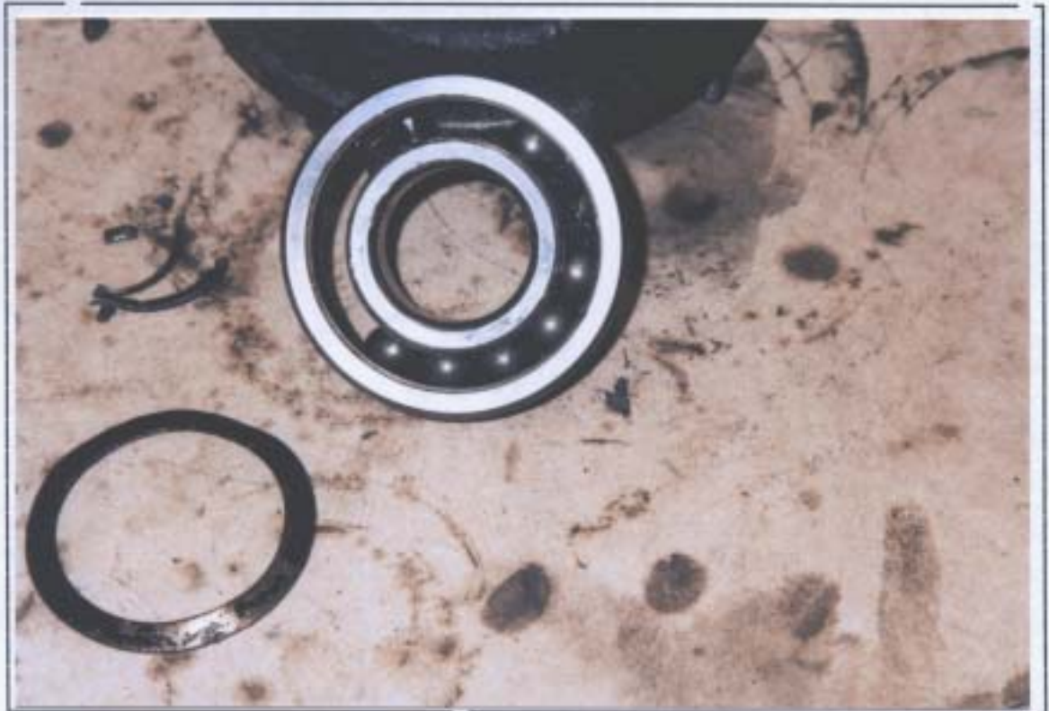
Fig 6 View of Deep Groove ball bearing showing damaged ball race and cage.
