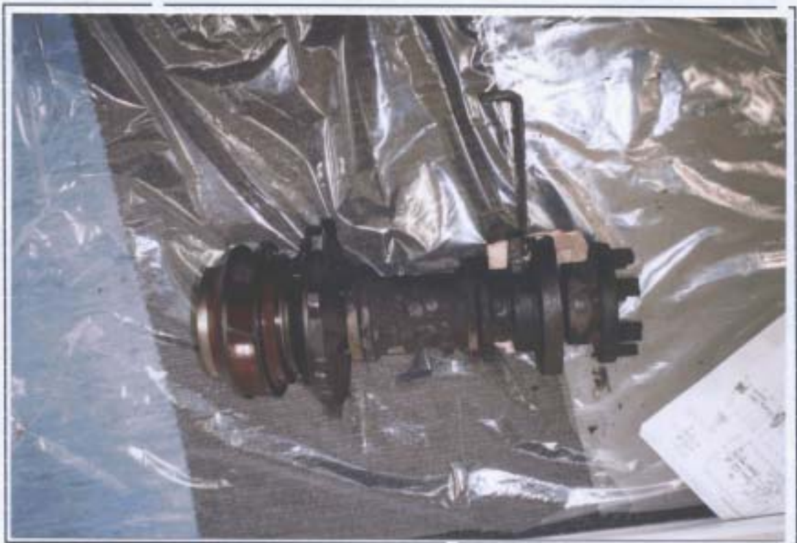
Fig 3 General view of shaft, impeller, bearing bracket, and drive coupling before being stripped for inspection.
