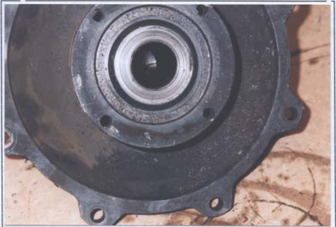
Fig 4 Close-up view of discharge cover showing heavy face plate wear caused by movement of shaft forward and contact between thrower and discharge cover.
