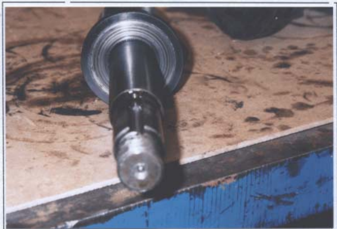
Fig 5 Close-up of impeller shaft thrower showing corresponding wear pattern.
