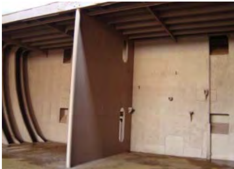
Figure 2 – Photo of MV SWANLAND Hold, Showing Longitudinal Bulkhead at Fr24-31
