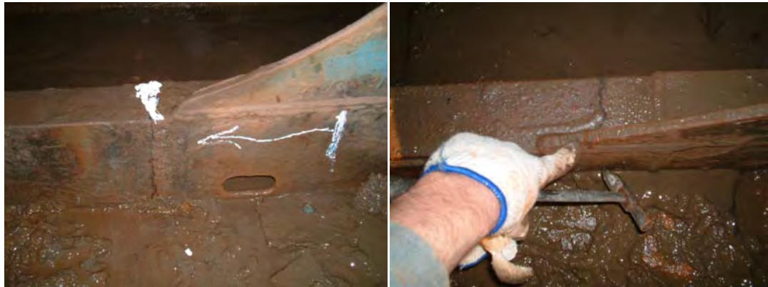
Figure 8 - Examples of Cracks in Bottom Longitudinal Members (Not MV SWANLAND)
