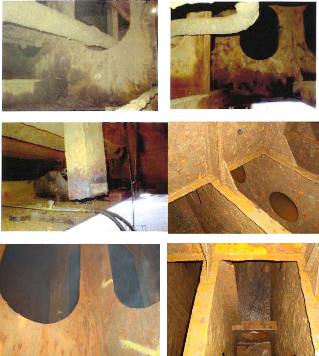
Figure 11 – Various Photos of Double Bottom Tanks Showing Heavy Corrosion and Wastage (2009, exact locations unknown)
