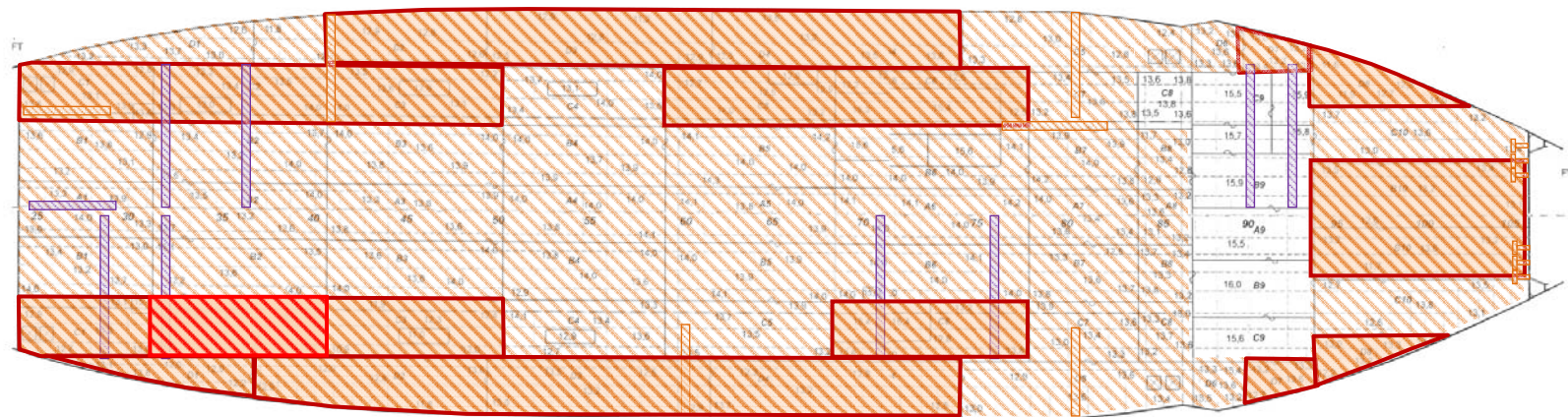
Figure A.3(d) – Tank Top Plating Areas Renewed at 2009 Dry-docking and Areas of Diminution Greater than 15%
