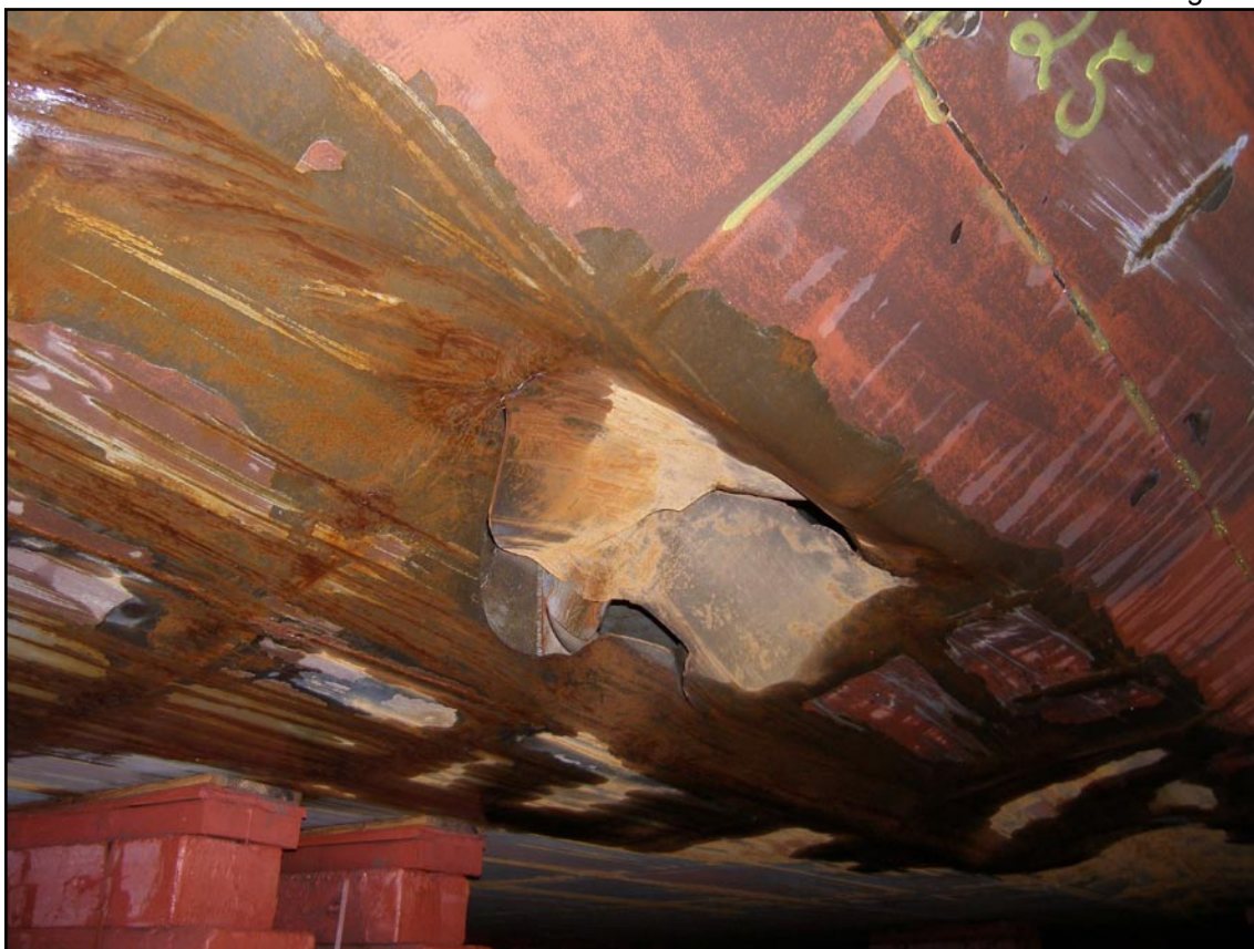
Damage to port side no. 3 water ballast outer tank
