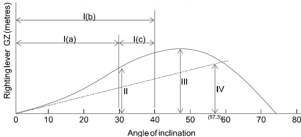
Diagram 4 – Example of righting lever curve with requirement key points
