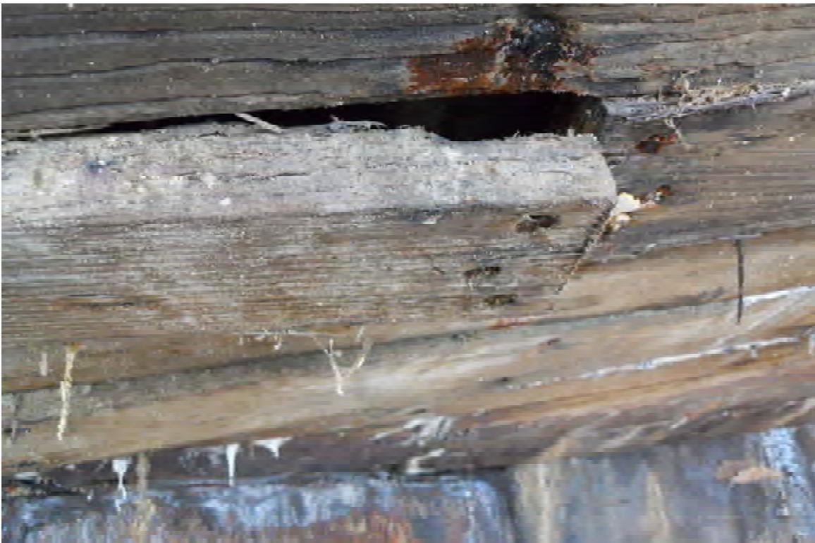
10 - Plank 7 starboard side sprung at butt.JPG
