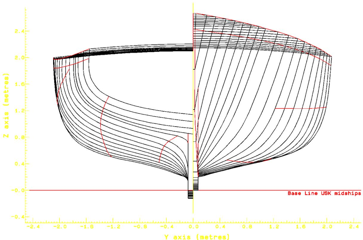
Diagram 1 – Hull sections
