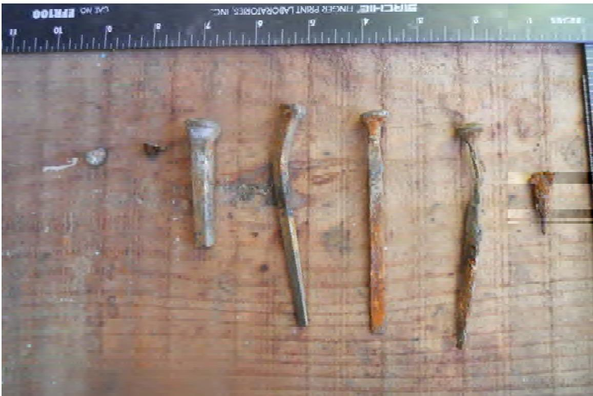
12 - Fastenings removed from starboard side of hull.JPG
