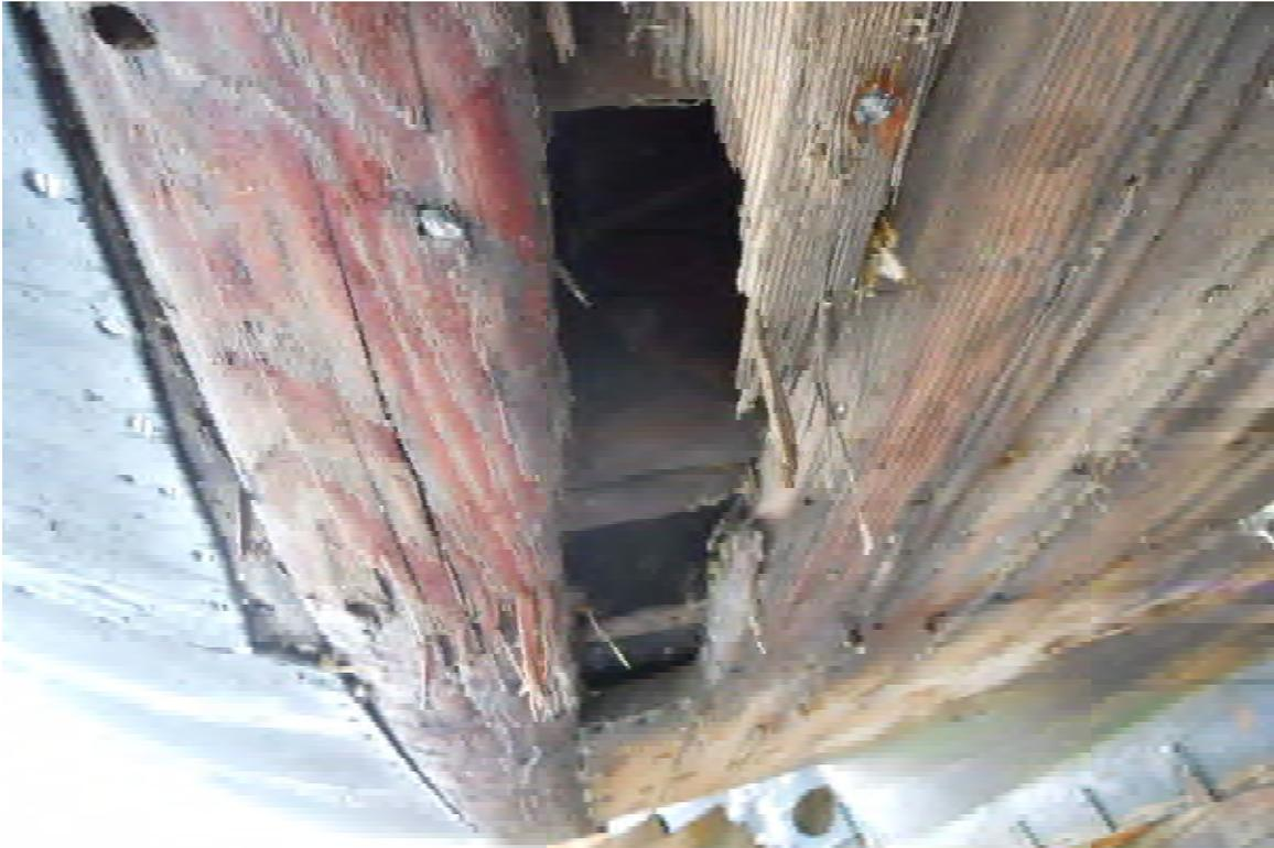
9 - 9th plank out from keel starboard side with section missing.JPG
