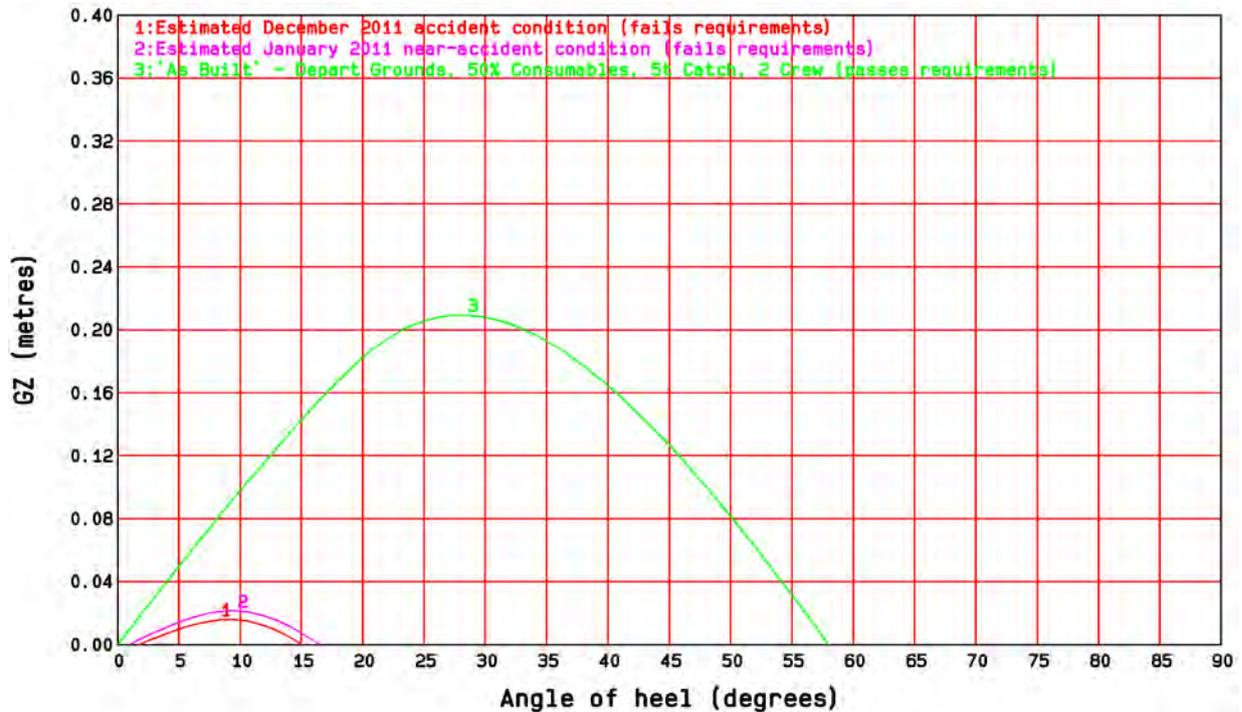
Diagram 6 – Righting lever curves for the 2011 accident, near accident and Depart Grounds ‘As built’ conditions
