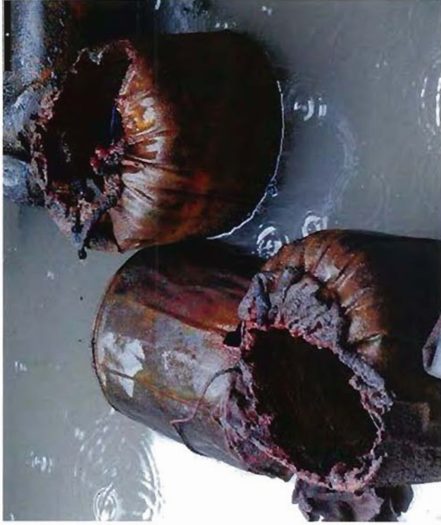
Photograph 45 The burnt 25 litre drums in the Steering Gear Room
