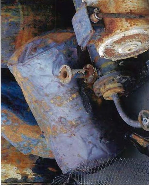
Photograph 51 A 200 litre drum with creased sides which has subsequently over-expanded
