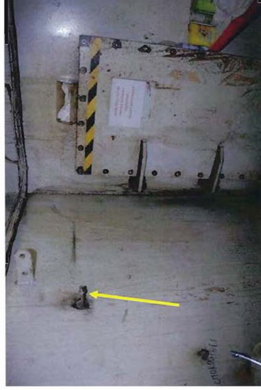
Photograph 24 The retaining bolt on the bulkhead to keep the access door to the Engine Room Workshop open at sea
