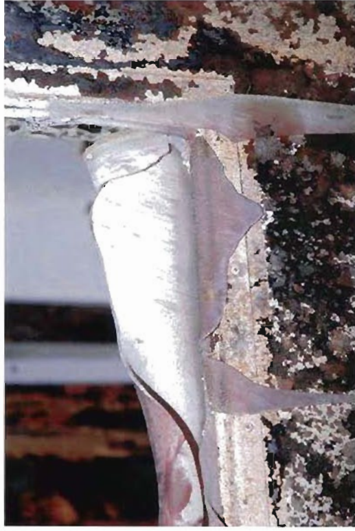
Photograph 41 The resolidified glass in the window of the door to the Engine Control Room
