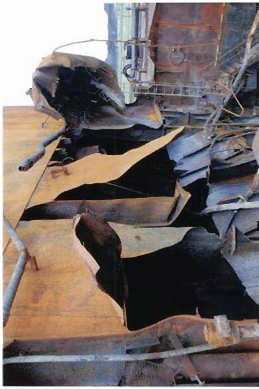
Photograph 9 The damage to the aft bulkhead of the Engine Room
