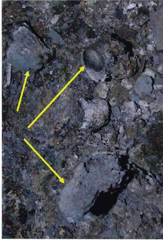
Photograph 17 Resolidified melted steel adjacent to the Diesel Oil Service Tank
