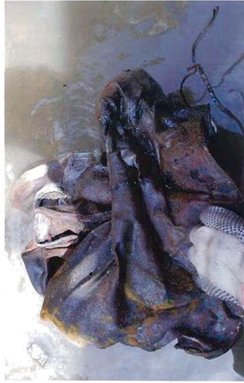
Photograph 54 The remains of a severely crushed 200 litre drum between the rudder head and the transom
