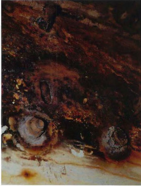
Photograph 29 The severely rusted nuts on the retaining bolts for the "Hardox" tiles
