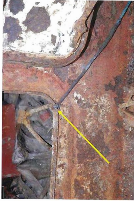
Photograph 6 The remains of a welding cable through the door of the Deck Workshop
